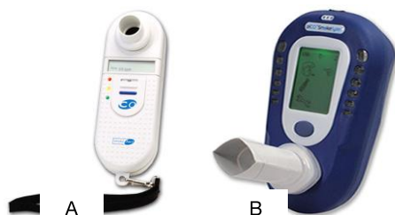
Figura 2: A – Micro CO/Smoke Chek ; B - piCO+ Smokerlyzer .
